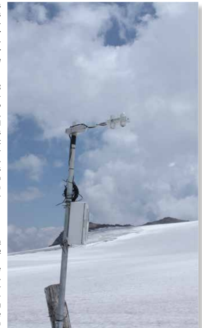
Fig. 1 - A net radiometer installed at the surface of the Cevedale Glacier to sample energy fluxes in order to calculate surface albedo. Albedo data have been analyzed with respect to BC concentration values.
