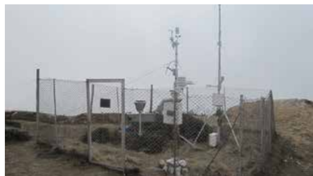
Fig. 2 – AWS QC and AWS Namche installed at 3570 m a.s.l. (Nepal). The comparison activity was carried out from 11 May to 21 June 2013.
