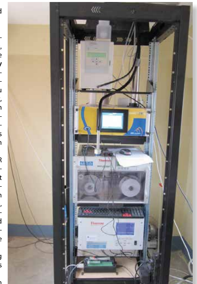
Fig. 2- Internal view of the SusKat station at Pakanajol: condensation particle counter, OPC, MAAP and ozone analyser.
