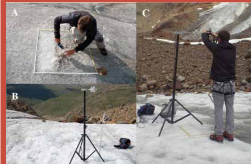
Fig. 4 - Series of pictures illustrating: (a) sampling supra-glacial debris, (b) measuring albedo and (c) acquiring high resolution digital images of the glacier surface.
